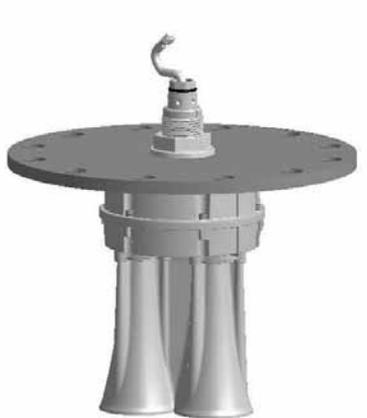
Figure 8 Screw Nut onto the Neck Tube
