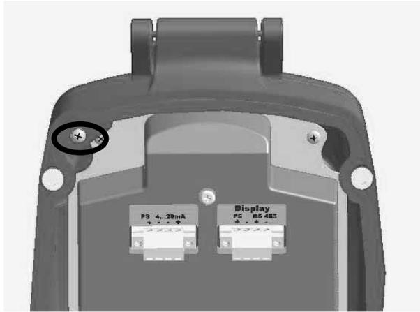
Figure 34 Internal Ground Terminal
