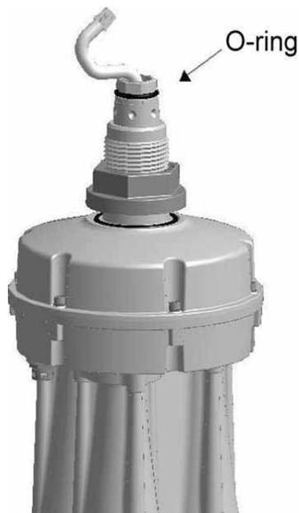
Figure 5 Neck Tube O-Ring
