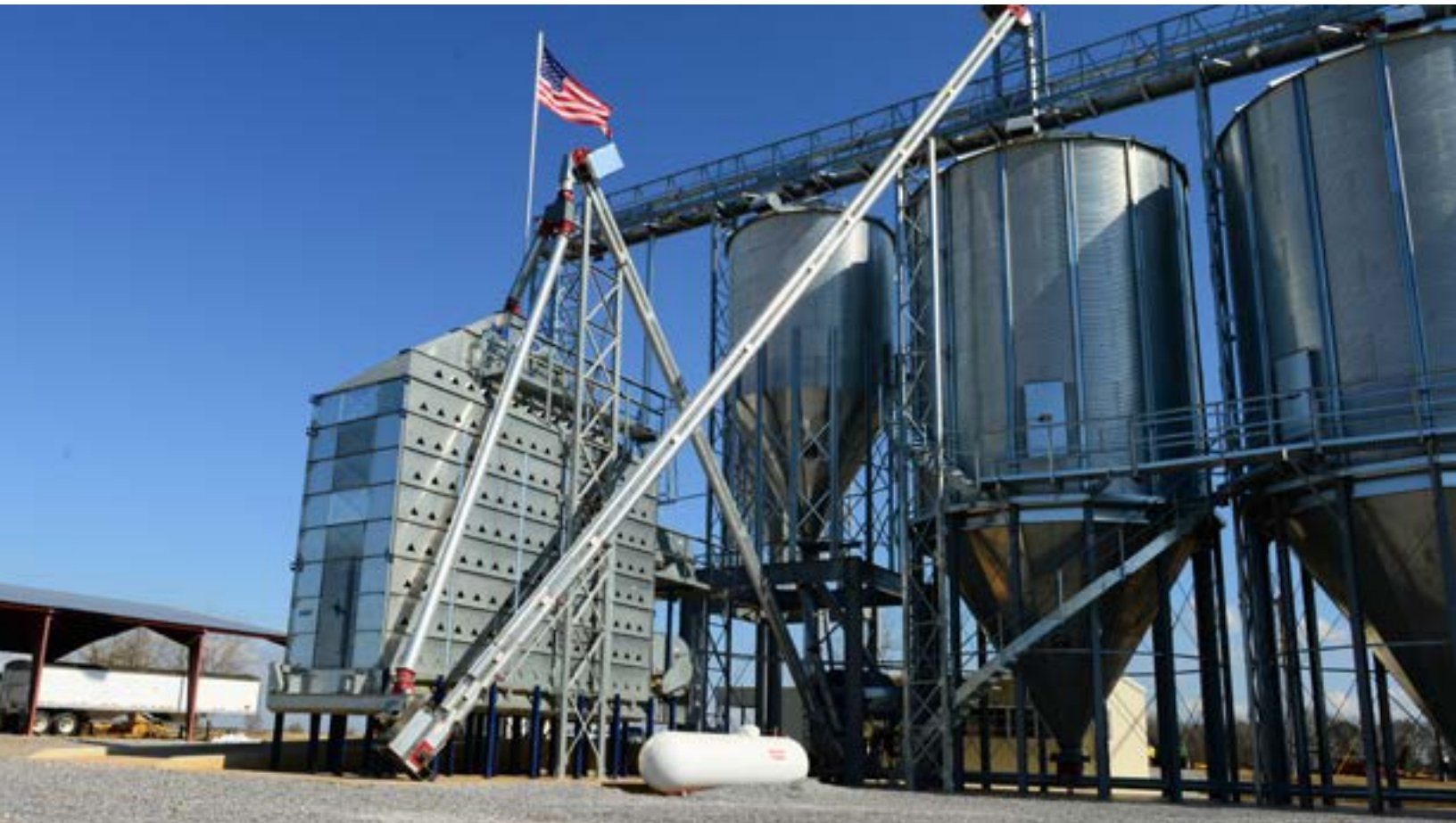
Stationary Double Run filling a dryer and unloading dryer to multiple bins.
