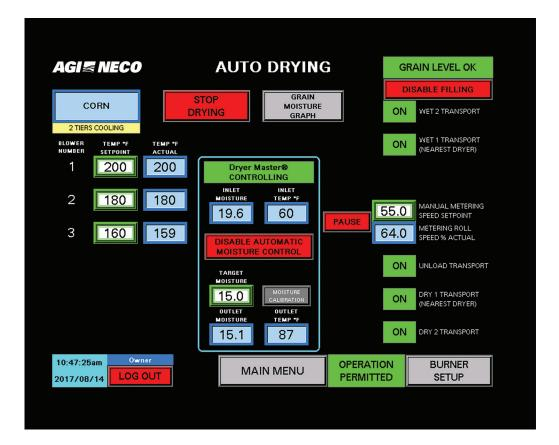
DRYER MASTER provides high quality moisture control in the industry. DRYER MASTER's model based moisture control technology is embedded in NECO's control panel, which is a NECO EXCLUSIVE. Dual moisture sensors provide the information required to deliver accurate, consistent moistures, reduce over and under drying, maximize throughput and lower energy consumption.
