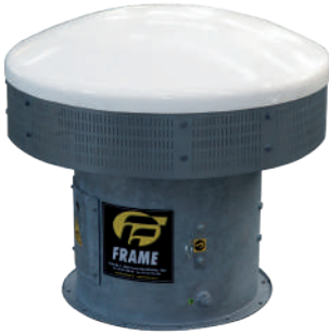
TORXEF504X2 Powered fan 0,75 kW, Volume: 8,000 m 3 /h @ 5mm swg – ATEX 22
