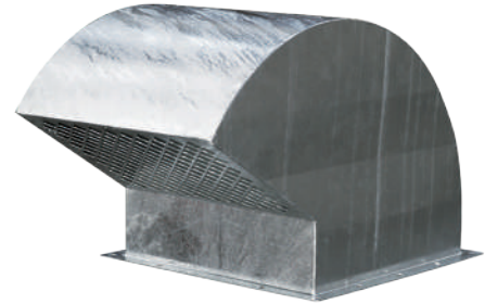
AERAP-XM Curved roof vent, with powered fan 0.18 kW, Volume: 2,000 m 3 /h @ 5mm swg – ATEX 22. Curved roof vent, included as standard on all silos above FP 18. As an option, remotely operated louvres are available for roof vents when fumigating the silo
